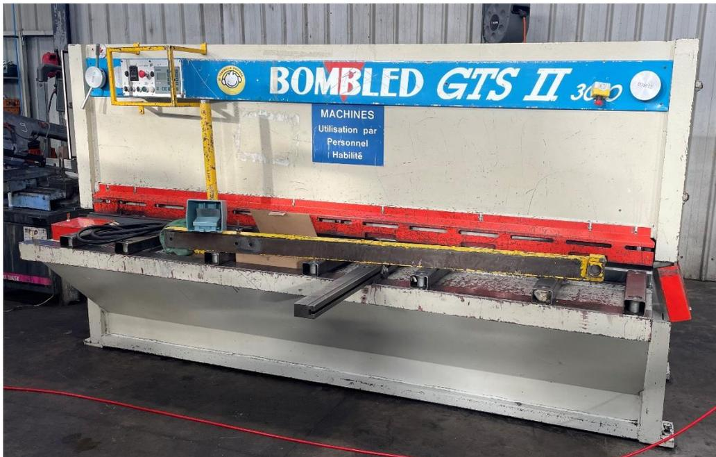
Cisaille hydraulique BOMBLED GTS II
