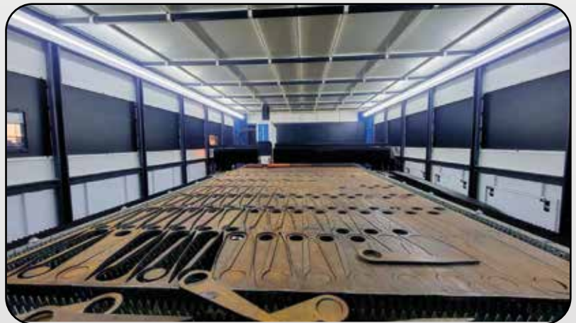
SF Laser 6 x 2,50 m - 12 kW
